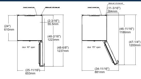
Allow door swing clearance at locations next to a wall. If the appliance is installed with the hinges next to a wall, the distance between the appliance and the wall must be at least  $1\frac{1}{2}$ " (40 mm). This is how far the handle protrudes when the door is open.
