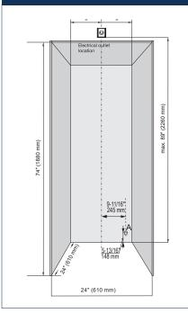
The appliances can be used freestanding or semi built-in. If semi built-in, consider the minimum cabinet opening dimensions specified on this image. For ventilation requirements, please follow instructions on section Ventilation Requirements in the Freestandig Design Guide.
