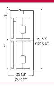
The first step of the installation is measure the current cutout dimensions and compare them to the cutout dimensions shown below. Little or no cabinet work may be necessary.
