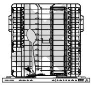
Ensure large utensils are not jammed against the door as this may stop the detergent dispenser from opening.
