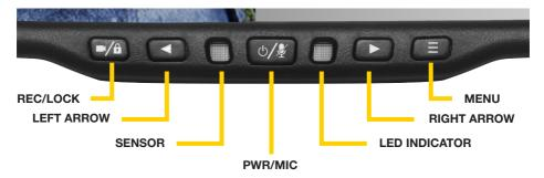
Pressing the menu button when a video signal is being viewed will allow you to adjust the following parameters.
