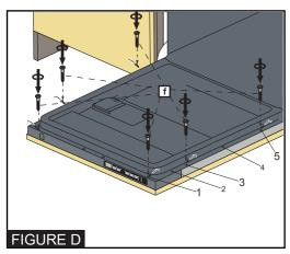
7- As shown in Figure D, Screws Ø 5/32" x 53/32" (Ø 4mm x 42,5mm) are installed in positions I,III and V.
