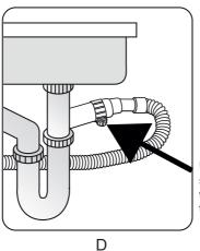
Use hose clamp shown in Figure D. for drain hose assembly to the sink.
