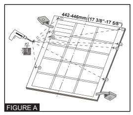
1. The mounting plan in the plastic bag is fixed to the inside of the Dishwasher door.
