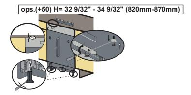
If the height of the enclosure is above 34 9/32" (870mm) use long supports as shown in the figure.
