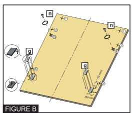
3- As shown in Figure B, Screws  $\emptyset$  5/32" x 27/32" ( $\emptyset$  4mm x 21,5mm) is installed in positions III.
