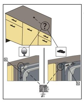
10- Mounting brackets previously fixed to the dishwasher are also fixed in the cabinetry with Screws Ø 5/32" x 19/32" (Ø 4mm x 15mm).
