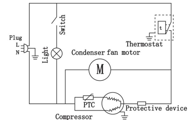
Note: This wire diagram is just for reference only. The wiring label on back of refrigerator will be accurate.
