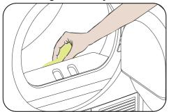
Inside the machine, there are humidity sensors that detect whether the laundry is dry or not.
