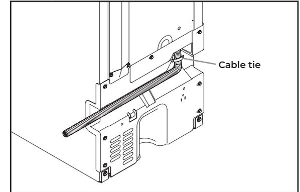
**15** Using a cable tie, fix the drain tube to rear panel as shown in the illustration.
