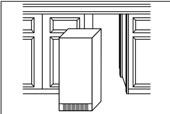
**3** If ice maker is built into cabinets, pull ice maker out of the opening.
