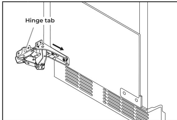
**2** Take the original top hinge, flip it and place it in the bottom hinge position on the opposite side. Slide onto the cabinet hinge screws. The hinge tabs on the hinges should always face towards each other.
