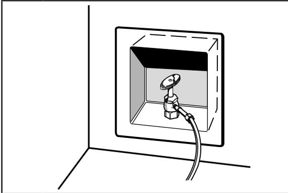
**2** Turn off water supply. Wait 5 to 10 minutes for the ice to fall into the storage bin. Remove all ice from bin.
