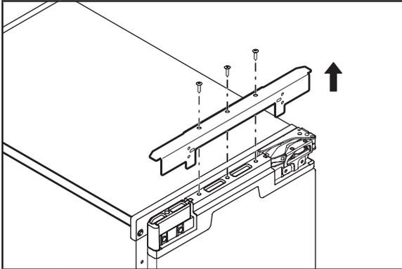
**2** Remove the screws and the top metal bracket using the Phillips screwdriver. Place them aside.
