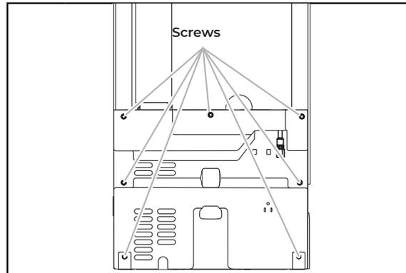
**1** Unscrew the screws attaching rear panel to ice maker. Remove the screws and rear panel, place them aside. For pump models, skip to step 12.
