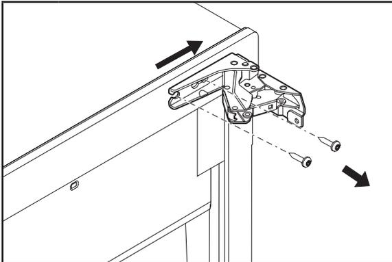
**7** Remove the screws and hinges from the cabinet with the Torx T25 screwdriver and place them aside.
