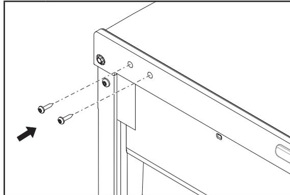
**1** Install the hinge screws (placed aside in step 7 of "Preparing the Bottom Hinges") half way on the desired side of the cabinet.
