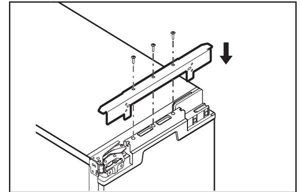
**3** Reinstall top metal bracket using screws removed in the step 1.
