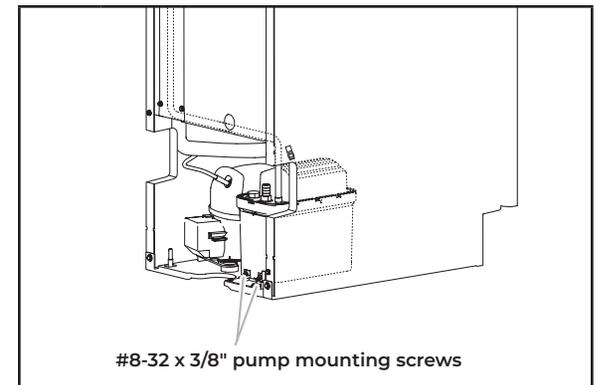
**4** Align the two screw holes at the rear of the pump. Use the two #8-32 x 3/8" screws supplied to attach the pump to the ice maker base.
