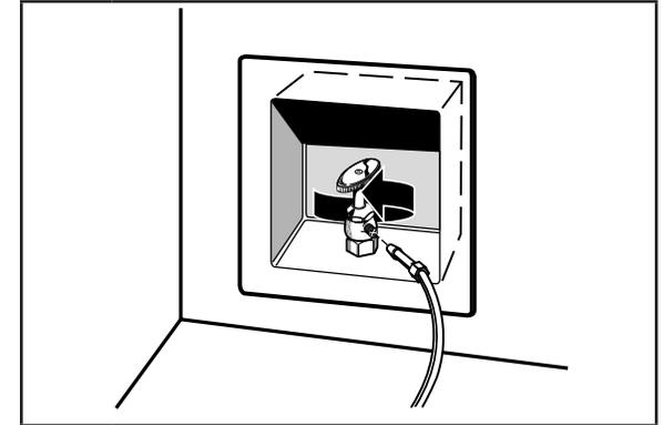
**7** Turn shutoff valve on. Check for leaks. Tighten any connections (including connections at the valve) or nuts that leak.
