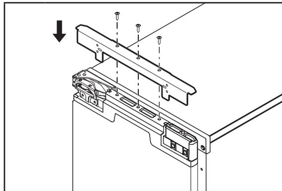
**8** Reinstall the top metal bracket on the door.
