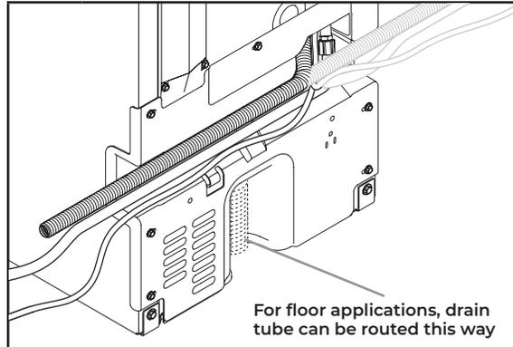
**14** Route the drain pump discharge tube, power cord, and water inlet through the slot in the ice maker back panel. Replace the rear panel and screws.
