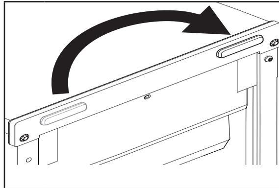
**8** Remove the screw cap cover and replace on the other side.
