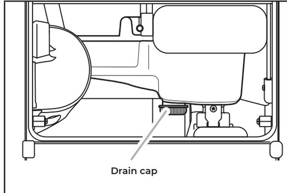
**4** Unscrew the drain cap from the bottom of the water pan located inside the storage bin. Allow water to drain completely.
