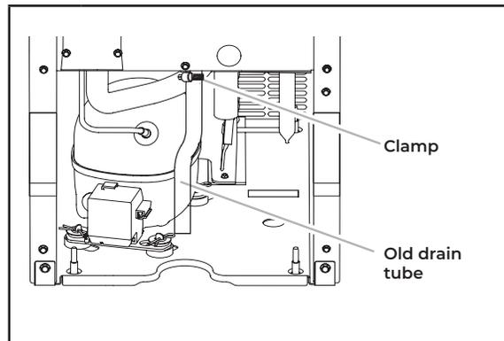
**2** Remove the old drain tube and clamp attached to the ice maker bin.
