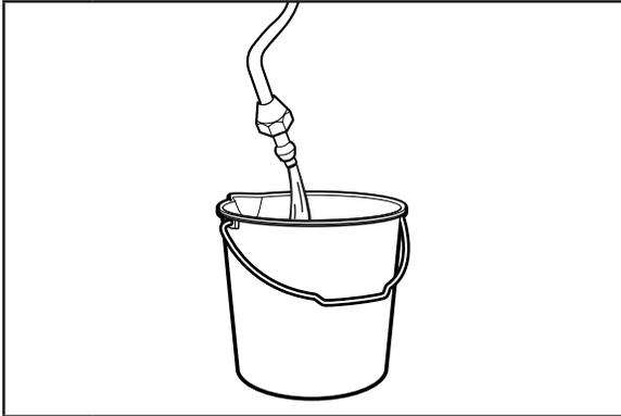
**4** Flush out tubing by placing the free end of the tubing into a container or sink, and turning on the main water supply until water is clear. Turn off shut-off valve on the water pipe.
