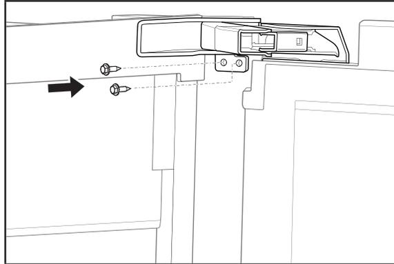
**7** Be sure that the ice maker is at desired depth. Secure the top and bottom hinges to the side of the cabinet using wood screws.
