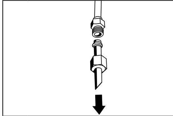
**5** Remove and discard the short, plastic tube from the end of the water line inlet.
