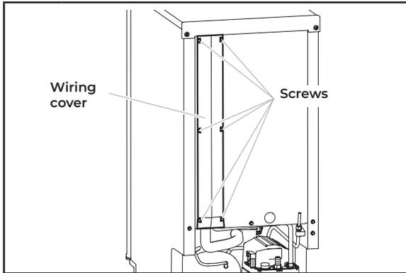
**5** Unscrew the screws attaching wiring cover to the ice maker and remove the wiring cover. Place the screws and wiring cover aside.
