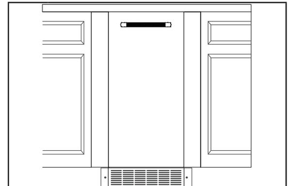
**6** Using the TORX T20 screwdriver, screw auxiliary grill into cabinet.
