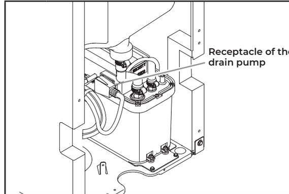
**9** Coil the ice maker power cord into a 4" (10.2 cm) diameter coil. Restrain the coil with electrical tape or cable ties. Place the coiled power cord as shown in the illustration and plug it into the receptacle on the drain pump.
