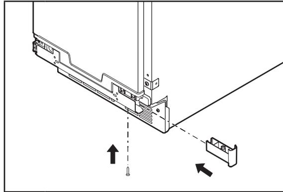
**7** Reinstall the top and bottom end caps on the door (the top right end cap is now the bottom left end cap and vice versa).
