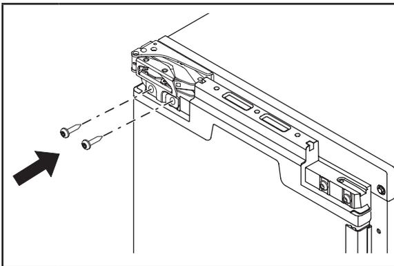
**6** Slide the door onto the hinges. Using Torx T25 screwdriver install the screws (removed in the step 6 of "Removing the Hinges" section) onto the door.
