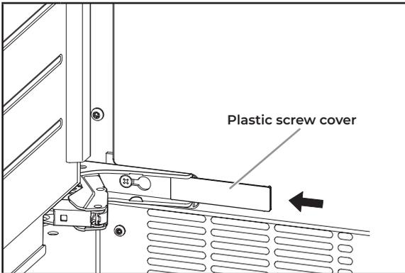
**5** Reinstall the plastic screw cover to original locations on the hinges.
