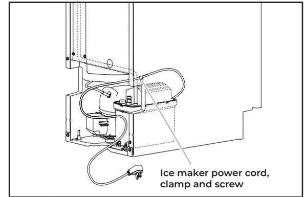
**8** Unscrew and remove the power cord clamp mounted to the ice maker side wall from the ice maker power cord.
