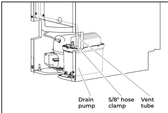
**6** Install vent tube [5/16" I.D. x 32" (81 cm)] to drain pump reservoir vent. Use one of the supplied 5/8" small adjustable clamp.
