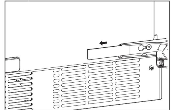
**6** Remove the plastic screw cover from the inside of the hinges and place them aside.
