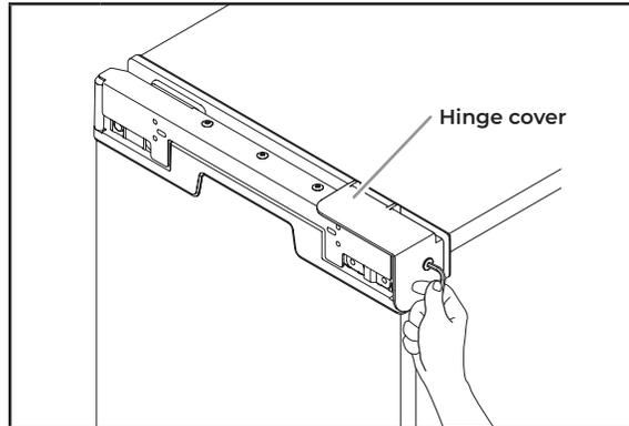
**2** Remove the screws attaching top and bottom hinge covers using an  $3/16$ " hex driver.
