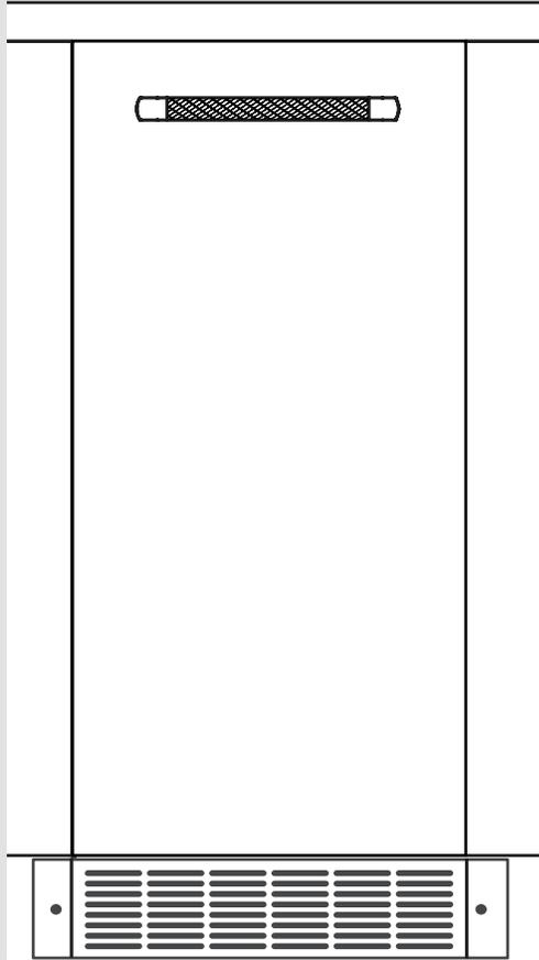
The auxiliary grill is an optional accessory. It can be used to align the toe grill with the rest of the cabinets (while not obstructing ventilation of the ice maker).
