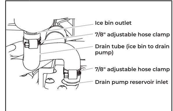
**11** New drain tube is provided in the drain pump kit. Install new drain tube to both the ice bin outlet and the drain pump reservoir inlet using new adjustable clamps.
