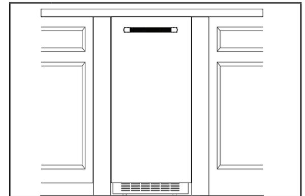
**4** Lightly press the custom panel onto the door using double sided adhesive tape. Adjust height of the panel to align with the adjacent cabinetry. Press the panel firmly against door.
