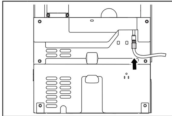
**6** Insert end of tubing squarely into outlet end as far as it will go. Screw compression nut onto outlet end with adjustable wrench. Tighten the nut by hand. Then tighten it with a wrench two more turns. Do not overtighten.
