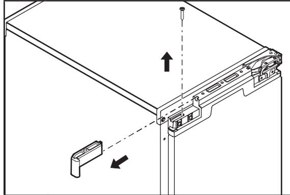
**3** Remove the screw from the top and bottom end caps using the Phillips screwdriver. Remove and place them aside.
