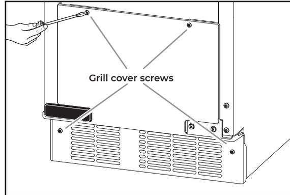
**1** Unscrew and remove the grill cover using a TORX T20 screwdriver. Place them aside.
