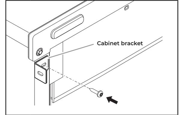
**8** Attach the cabinet brackets (provided with ice maker) to the holes in the front of ice maker as shown in the illustration. Attach the cabinet brackets to the side of the cabinet with wood screws.
