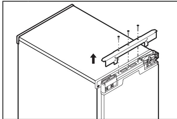
**1** Remove screws and the top metal bracket using the Phillips screwdriver. Remove and place them aside. Skip this step and go to the step 4 if the door reversal has been completed.
