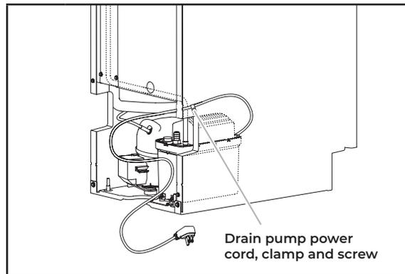
**10** Attach the drain pump power cord to the ice maker side wall with the clamp and screw (removed in step 7).
