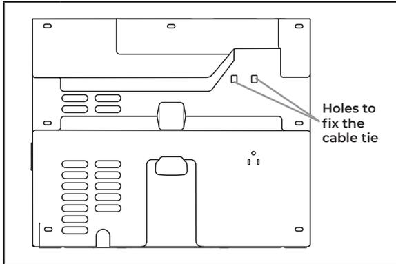
**13** Install the cable tie on the rear panel using two holes provided on the rear panel.
