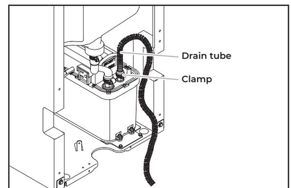
**12** Attach the drain tube to pump discharge tube using a clamp provided.
