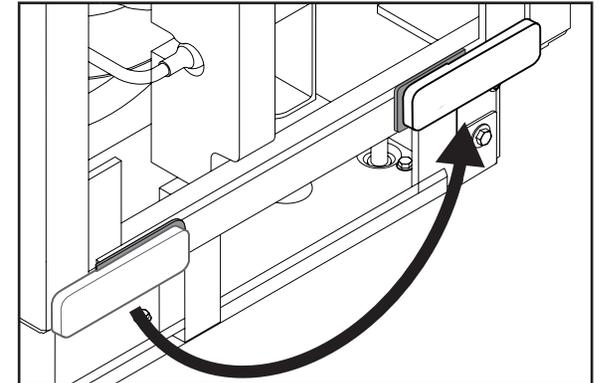
**2** Remove the screw cover and place it on the other side as shown in the illustration.
