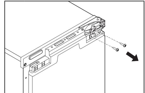
**4** Using Torx T25 screwdriver unscrew the door hinge screws completely from the top and bottom hinges and place them aside.
