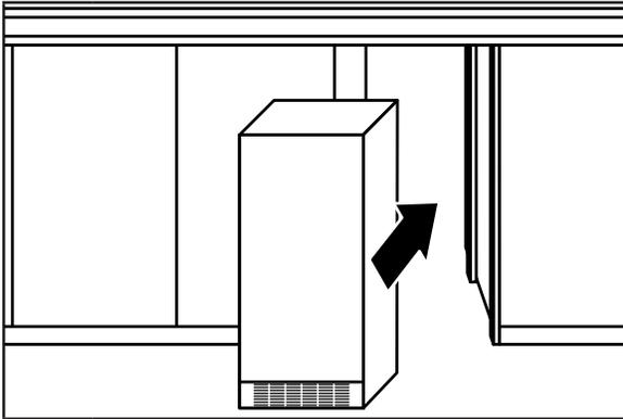
**6** Slide ice maker into the cabinet while managing the utility connection positions behind the ice maker. Be sure to cover the floor with cardboard or hardboard to avoid damaging it. **IMPORTANT:** For the flush install, the ice maker utility connections must be routed out through the slot in the ice maker rear panel.
