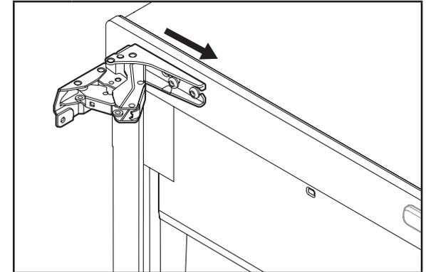
**3** Take the original bottom hinge, flip it and place it in the top hinge position on the opposite side. Slide onto the cabinet hinge screws.
