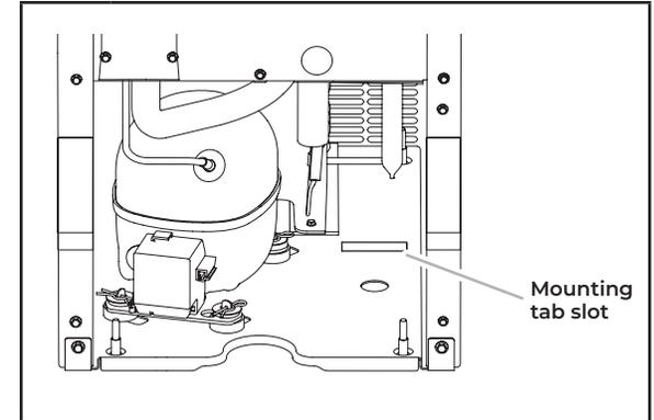
**3** Install the drain pump on the right side of the ice maker base. Tip the drain pump slightly to slide the mounting tab into the mounting tab slot.
