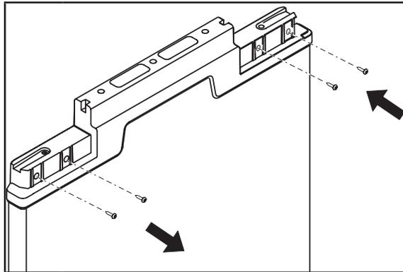
**5** Remove the door and place it aside. Swap the hinge screws to the opposite side.
