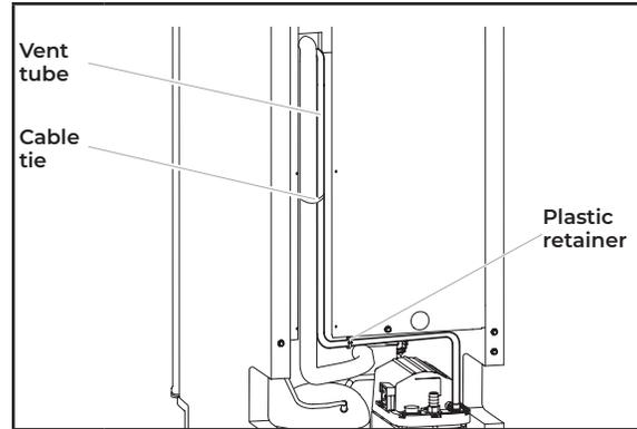
**7** Route the vent tube through the plastic retainer as shown in the illustration. Using a cable tie, tie the vent tube to the suction tube and wires located behind the wiring cover. Reinstall the wiring cover and screws.
