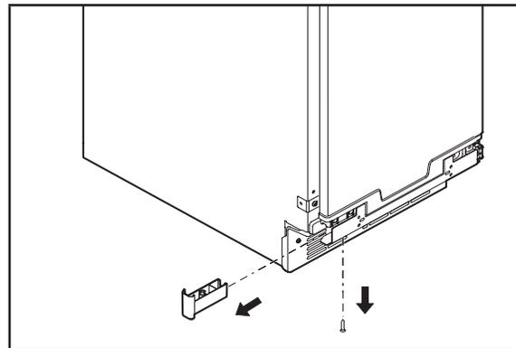
**2** Remove the top and bottom end caps using the Phillips screwdriver and place them aside.
