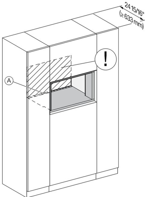
A - Cut-out (4" x 28" [100 mm x 720 mm]) in the bottom of the cabinet for the power cord and Ventilation
