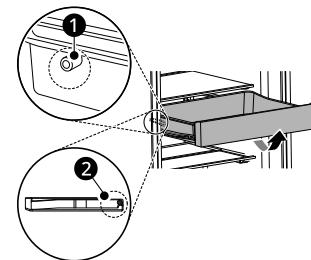
**2** Tilt the drawer slightly and support it with one hand while pulling it out.
