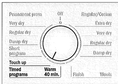
Time programs run at specific temperatures. Suitable for predried, multi-ply, delicate textiles or individual small items. Also for subsequent drying.
