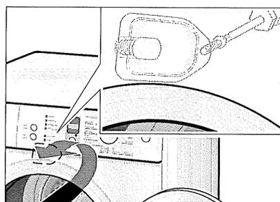
4. Loosen the screw of the cover and open the cover.
