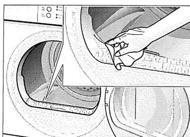
This deposit can easily be removed by wiping the sensors (the two bars next to the lint filter) with a cloth and a little white vinegar. Use white vinegar only! Clean the moisture sensor once a month.
