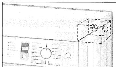
To connect the power cord you have to remove the cover plate.
