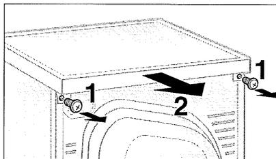
1. Remove the screws of the cover plate on the rear side of the appliance.
