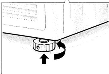
The dryer should be level with all four feet firmly on the ground. The dryer must not wobble.
