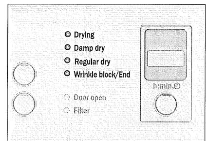
**i** At program end the LED "Wrinkle block/End" illuminates.
