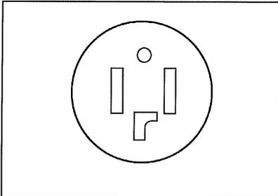
When installing the receptacle for the dryer cord, ensure that the power supply cord is accessible when the dryer is in the installed position.
