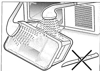
7. Clean the air cooler completely, drain thoroughly.
