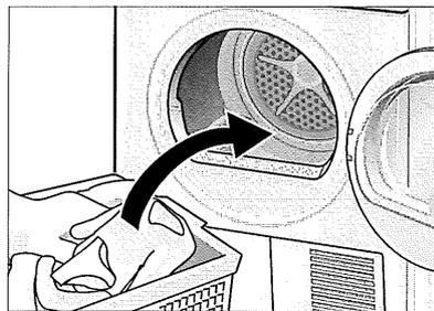
6. Place laundry in the empty drum. Put each piece of laundry into the machine separately. For best results the laundry to be dried must be sorted according to type of laundry and desired degree of drying. For further information see page 16.
