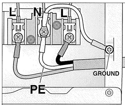
**i** Make sure that the U.L. strain relief clamp is outside the cover!
