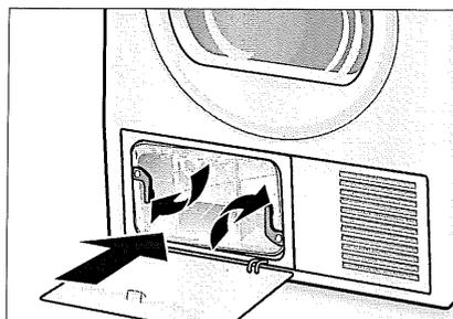
9. Re-insert the air cooler, handle at the bottom!
