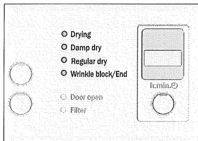
**i** If the indicator light "Wrinkle block/End" illuminates when the program selector is in Off-Position – turn off the circuit breaker and call for customer service!
