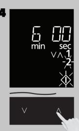
Set desired standing time by tapping " $\vee$ " / " $\wedge$ ". (up to 1 hour and 30 minutes).
