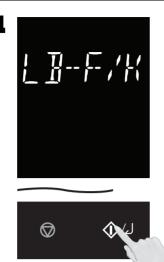
Touch **Start/Set** once. **"LB-F/KG-C"** scrolls across display window. The oven has a choice of Metric Units or Imperial Units display. The default weight unit is LB-F.
