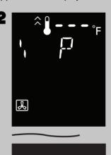
Touch **Start/Set** to preheat. "PREHEAT" will scrolls across display window once then a "P" will appear in the display window. When preheating is completed, the oven will beep and "P END" will display in the display window.
