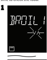
Touch **Broil** until the desired power level appears in the display window.
