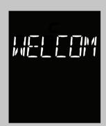
Plug into a properly grounded electrical outlet. "WELCOME TO PANASONIC REFER TO OWNER'S MANUAL BEFORE USE" scrolls across display window.
