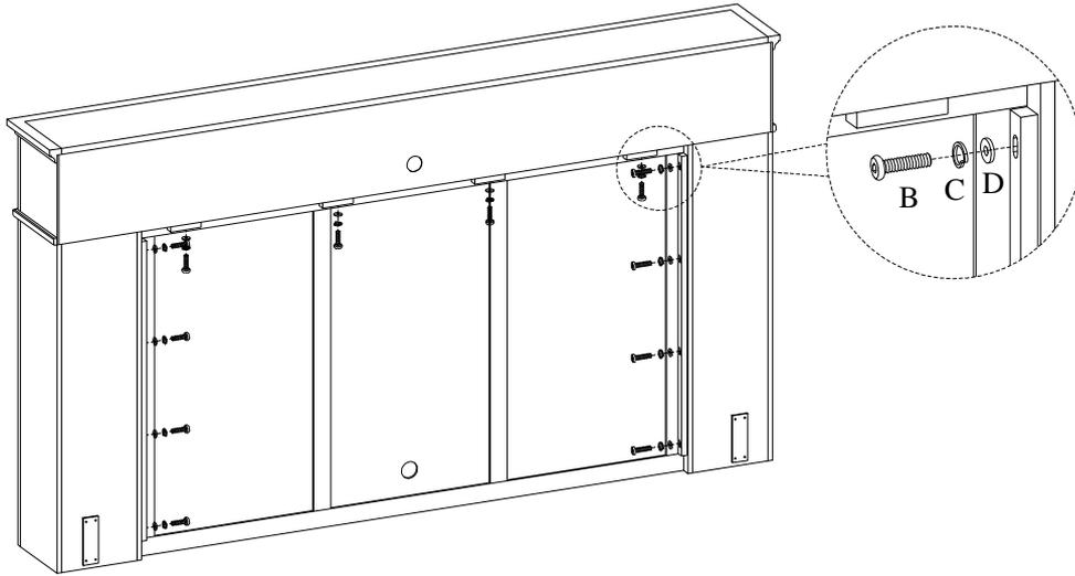
**STEP 5:** Place the hutch on the console. Take off one screw from each large metal plate on the back of hutch and swing it in an ideal location as shown below. Then re-secure the large metal plate with screws (G) to both hutch and console.
