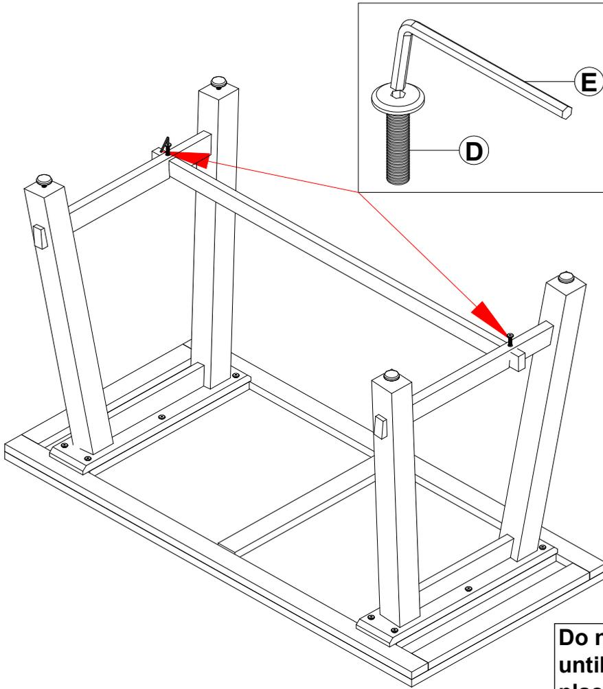
**Do not fully tighten until all screws are in place and properly aligned**
