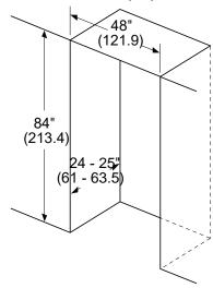
Leave ½" gap at the top and 1" behind the refrigerator for proper ventilation.
