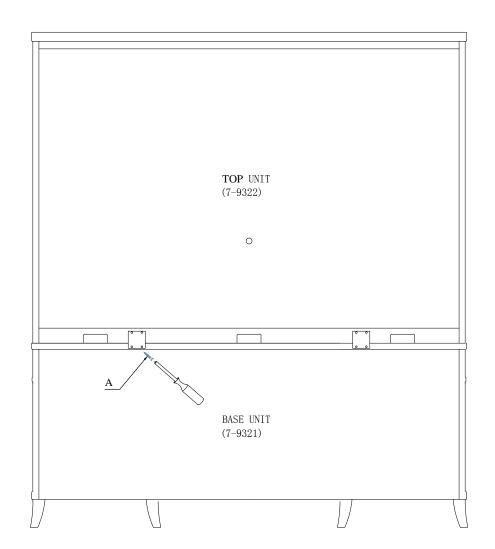
PLACE THE TOP ON THE BASE TOP, SECURE THE UNIT BY USING THE SUPPLIED MENDING PLATE AND SCREWS ON THE BACK.
