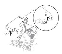
Remove the cover and pull out the tube (1). Disconnect all wire harnesses (2). Unscrew the ground wire (3).
