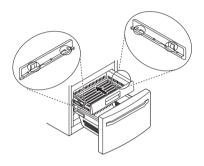
Replace the ice bin in the drawer. Insert the Durabase basket in the rail assembly.
