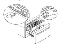
Remove the Durabase basket from the rails. Remove the screws from the rails at both ends.
