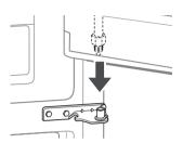
Fit the hinge (1) over the hinge lever latch and slot it into place. Rotate the lever (2) counterclockwise to secure the hinge.
