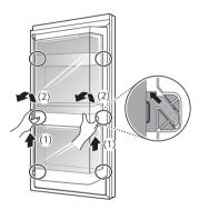
To replace the Door-in-Door case, line up the tabs on the Door-In-Door case with the slots on the door and push down until it snaps into place.
