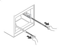
2 Grasp the drawer on each side and hook the drawer supports into the rail tabs located on both sides.
