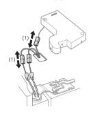
Rotate the hinge lever (1) clockwise. Lift the top hinge (2) free of the hinge lever latch.
