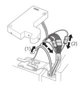
Rotate the hinge lever counterclockwise (1). Lift the top hinge (2) free of the hinge lever latch.
