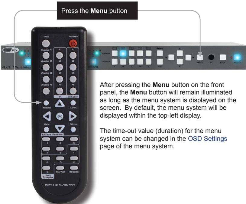
After pressing the **Menu** button on the front panel, the **Menu** button will remain illuminated as long as the menu system is displayed on the screen. By default, the menu system will be displayed within the top-left display.
