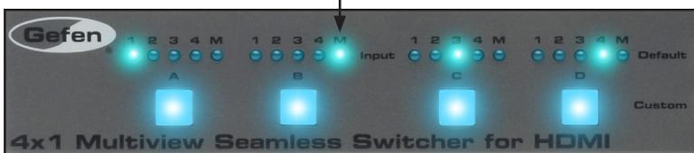
3. To unmask an window, press the button for the window and select the desired input.
