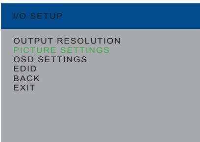
4. Press the **Select** button to display the **Picture Settings** menu. If using the IR remote, press the **OK** button.
