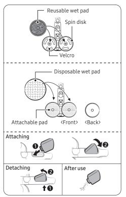
Use to clean a wooden or linoleum floor with a wet pad.
