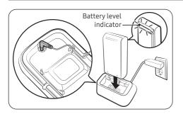
Charge the additional battery on the battery cradle.
