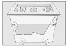
■ Using the large allen key, unscrew all four feet out by about 3/4" (2 mm).
