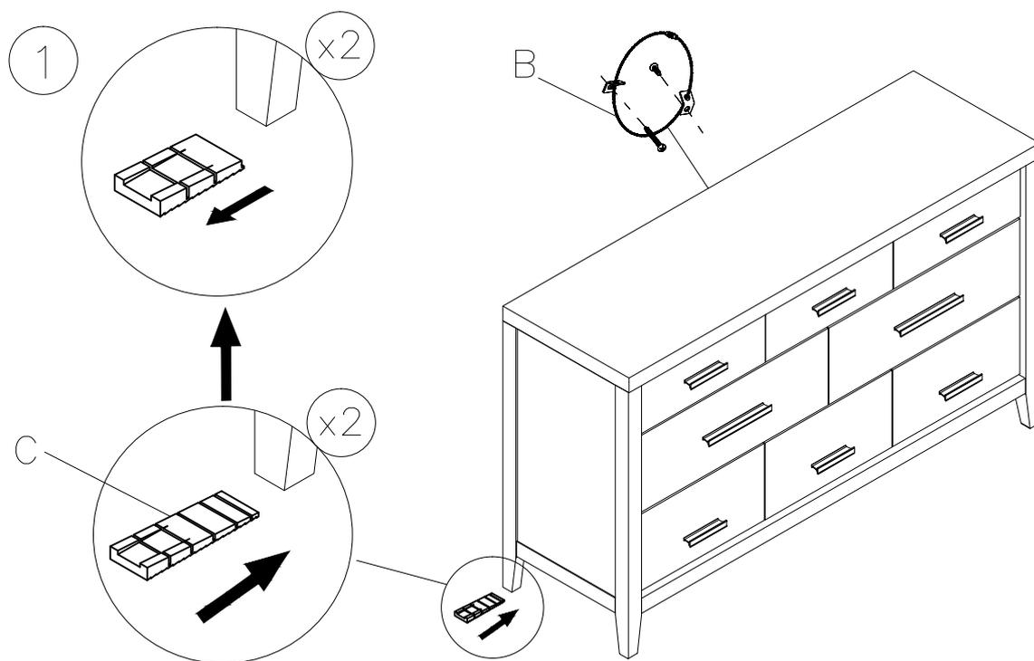
NOTE: IF THE UNIT IS PLACED ON AN UNLEVEL SURFACE, PLACE A LEVELER UNDERNEATH ONE FOOT UNTIL THE UNIT IS LEVEL. BREAK OFF ANY PROTRUDING SEGMENTS.
