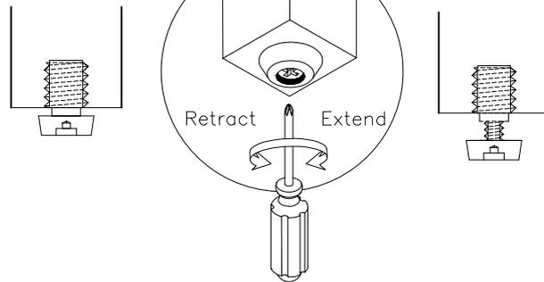
NOTE: Only use a hand tool screwdriver to adjust the leveler.
