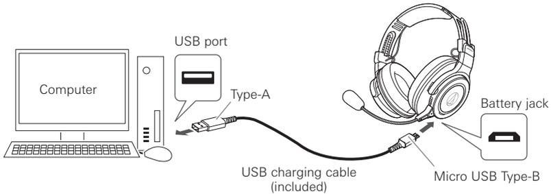
2. Connect the included USB charging cable (USB Type-A side) to the computer to start charging.
