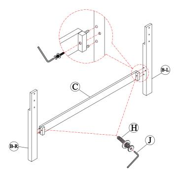
Attach Cross Bar (C) to Headboard Leg (L&R) (B) by using Bolt (H) and tighten with Allen Key (J).
