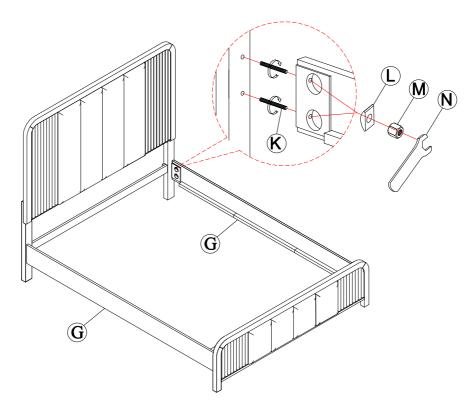
Attach Threaded Rods (K) to the Headboard and Footboard (D), then align side rail (G) to the threaded rods (K). Secure by using nuts (M) with Half moon nut (L).
