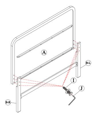
Attach Headboard Leg (L&R) (B) to Headboard (A) by using Bolt (I) and tighten with Allen Key (J).
