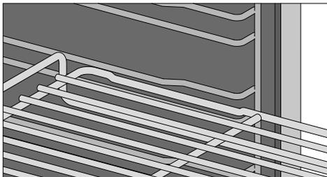
Always slide the wire oven rack into the rails on the shelf runner with the catches facing down.
