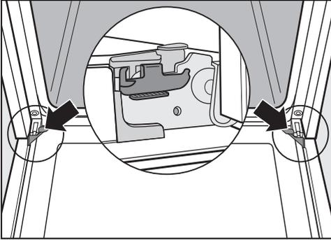
The oven door is connected to the hinges by retainers. Before removing the door from the retainers, the locking clamps on both hinges have to be released.
