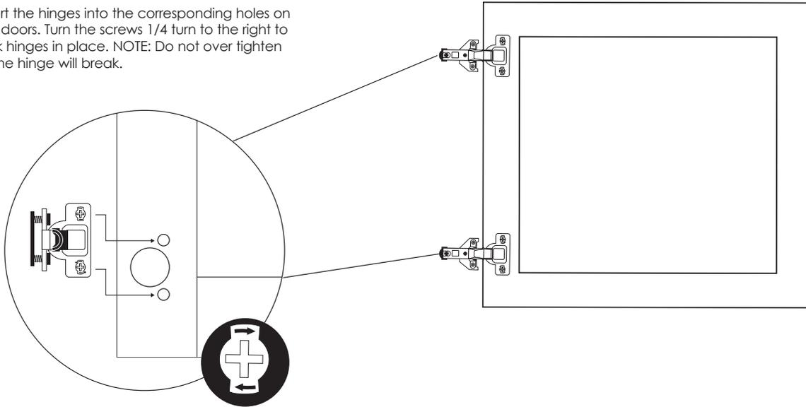
**Note:** The hinge can be separated by pulling the black tab and pulling apart the hinge from the hinge base. Separated hinges snap back together.
