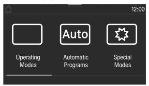
The menu path appears on the left of the **header**. The individual menu options are separated by a vertical line. ... I indicates that there are more menu options available if the menu path can no longer be displayed because there is not enough space on the display.
