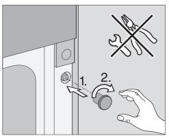
Screw the knurled nut onto the bolt by hand to fix the oven in the cabinet niche.
