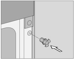
Insert the mounting aid into the hole in the front frame.
