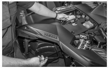
Take the speaker wire harness and run from the RFYXZ-K8 or RFYXZ-PMXDK harness under the hood to the holes drilled in the foot well.
