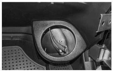
Attach the speaker wire harness connectors to the speaker terminals.
