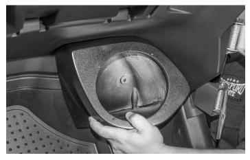
**Step 4 - Mount Speaker Enclosures** Remount the pod into the foot well location.
