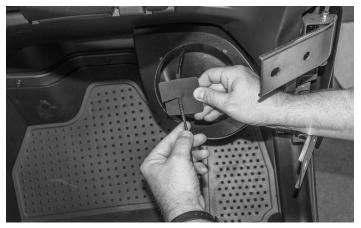
Apply the supplied foam sealing tape to the inside of the speaker enclosure to make sure you have a weather tight seal.
