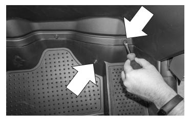
Remove the (2) bolts from the inside of the vehicle on both the passenger and driver's side.
