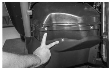
Remove the (2) spring nuts from the panels once the bolts are out of the way using a pick tool or small flat blade screwdriver.
