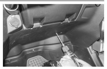
Remove the pod and drill (2) holes in the firewall using a 5/16" and 1/2" drill bit.
