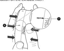
9 Push to insert the exhaust filter cover 3 into the exhaust filter 1 and rotate it to reassemble it and prevent it from falling out.
