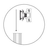
**B. Door Stops** Insert one left and one right door stop down center post.
