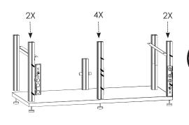
To ease installation of rear panels, gently place the unit face down on the floor to improve aligning of panels.
