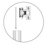
**C.** Top Door Hinges Slide the top door hinge plates through the front post channels, aligning with bottom door hinges.
