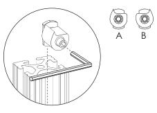
**D. Heavy Duty Bracket** Install heavy duty brackets down outer posts to support the double-width shelf. Place rubber shelf tabs through bracket.
