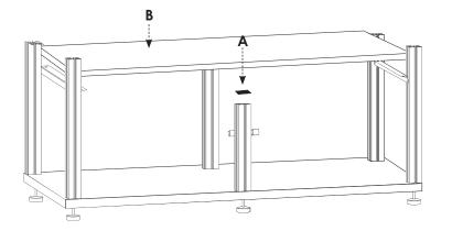
A. Rubber Pads Place rubber pad on top of center post.
