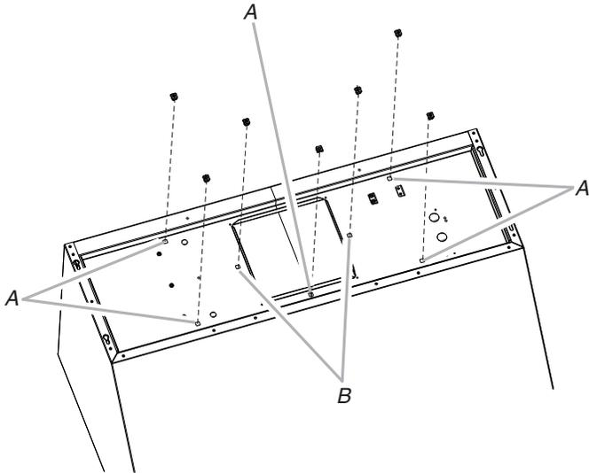
A. Clip nut locations for dual motor assembly (5)
