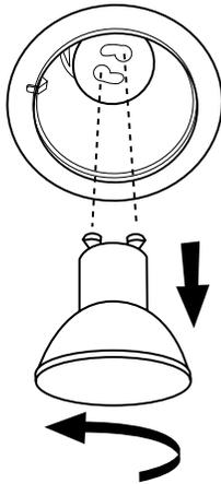
3. Remove the bulb and replace it with a 120-volt, 6.5 watt maximum LED bulb with a GU10 base. Turn it clockwise to lock it into place.
