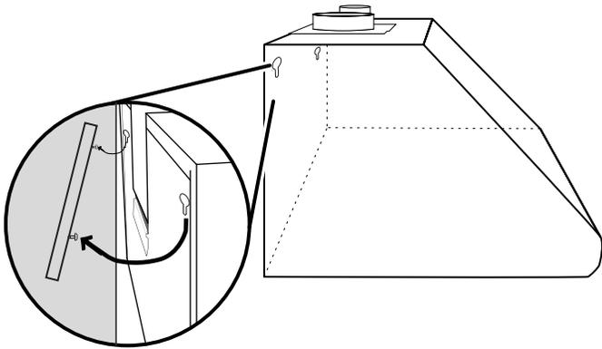
2. Push the range hood up into the narrow slots, align the bottom of the hood to the horizontal line, level the hood, and tighten the 2 mounting screws.
