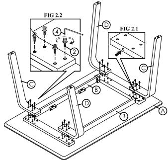
Step 2.1 Before assembling, please make sure table leg's hole for JCBB Bolt properly align to the Table Apron (B) as shown on FIG 2.1.
