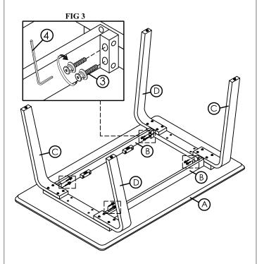
Step 3 Secure the Table Legs (C & D) to the Table Apron (B) using JCBB bolt and washer (3) and Allen Key (4) as shown on FIG 3
