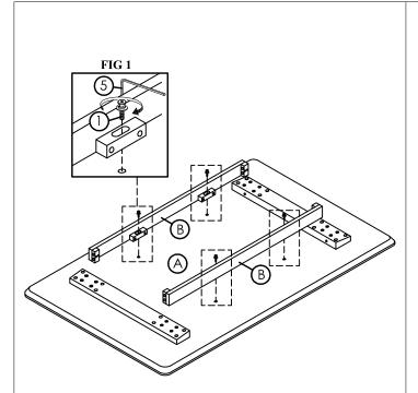
Step 1 Turn Table Top (A) upside down on a soft protective surface such as carpet. Attach Table Apron (B) to Table Top (A) using JCBC bolt with washer (1) and Allen Key (5) as shown on FIG 1.
