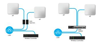
Access Point Placement: Place APs to ensure adequate coverage, but not so far apart that there is no signal overlap. You may have to experiment with AP placement to optimize the roaming experience. The APs should overlap enough that the client device has a good connection to the AP to which it is currently attached, but also sees the next-nearest AP.
