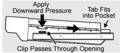
3. For removal, hold slide with one hand and lift drawer with the other to separate.
