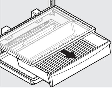
2. Apply pressure to drawer while supporting slide from below. Tab/clip passes through opening in drawer to locate. Ensure both sides are engaged.
