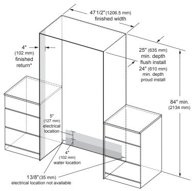
\*A minimum 4" (102 mm) finished return that matches the cabinet exterior is recommended on all sides and the top of the cutout opening. The shaded area will be visible after installation.
