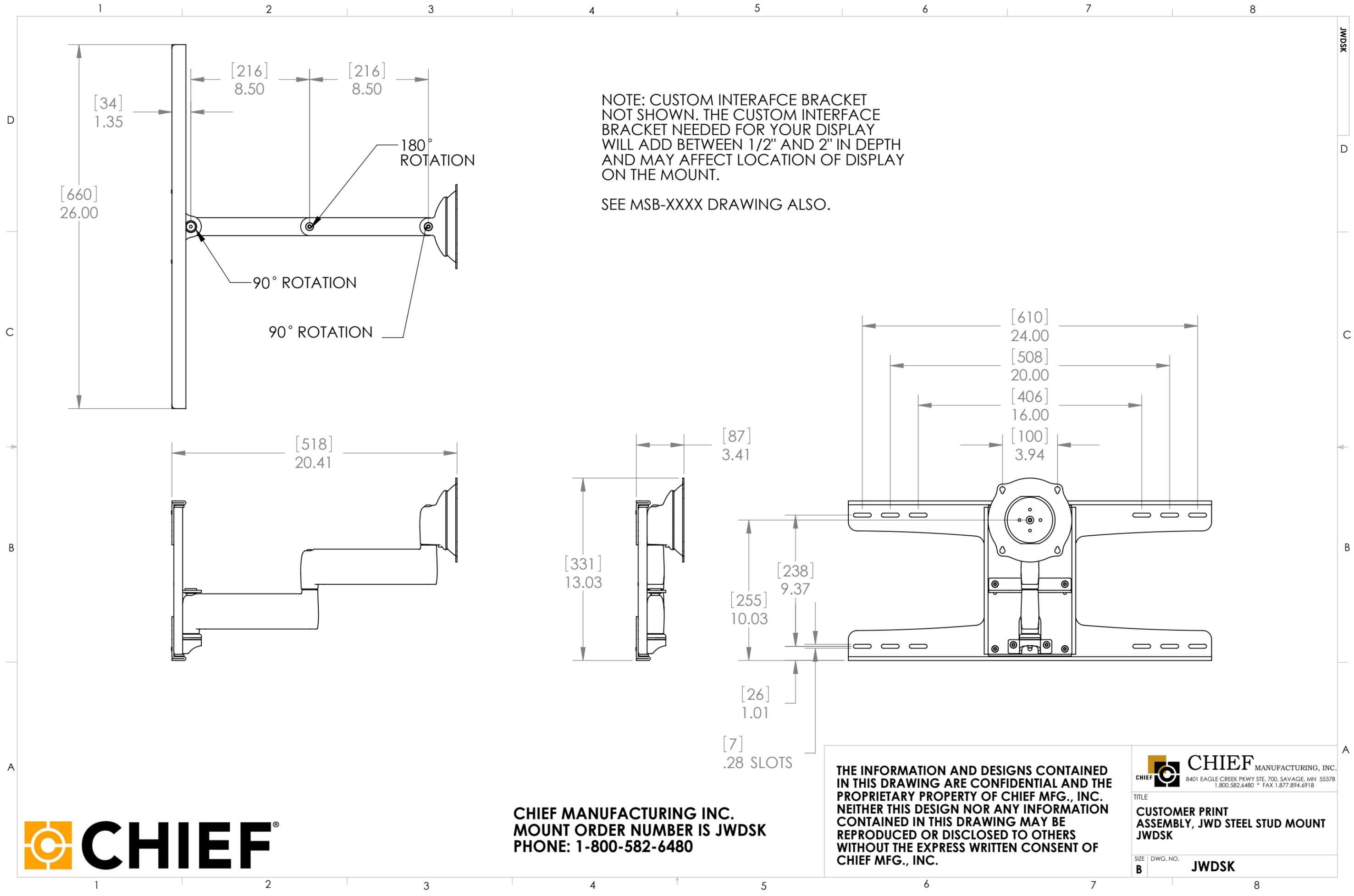
NOTE: CUSTOM INTERAFCE BRACKET NOT SHOWN. THE CUSTOM INTERFACE BRACKET NEEDED FOR YOUR DISPLAY WILL ADD BETWEEN 1/2" AND 2" IN DEPTH AND MAY AFFECT LOCATION OF DISPLAY ON THE MOUNT.
