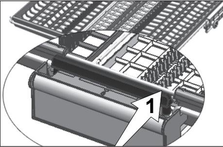
In models with partial movement feature, pushing the bar (1) on the handle enables the central tray of the basket to get to the lower position and the system gets unlocked. Thus right and left side trays can be used as moving parts.
