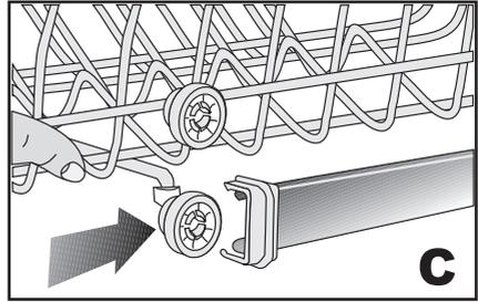
4. Push the latches back into the correct position.
