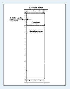
Do not restrict the air flow. The opening can either be directly over the appliance ①, above the cabinet and below the ceiling ② or through a vent installed in a soffit ③.
