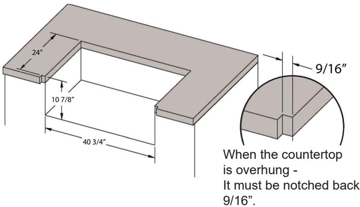
When installing, observe all clearances between the grill and adjacent structures as detailed in the Operating and Instruction manual.
