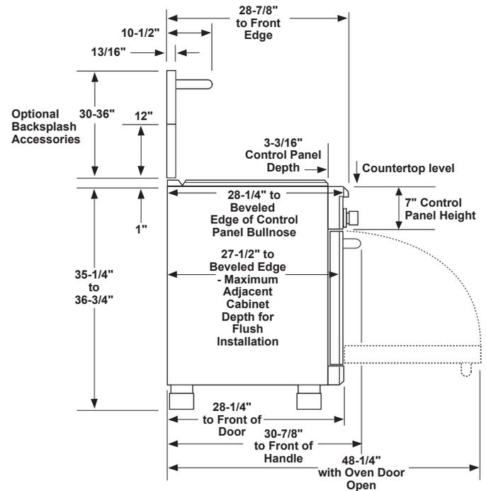
12" min. to combustibles or 0" to a non-combustible material above the cooking surface
