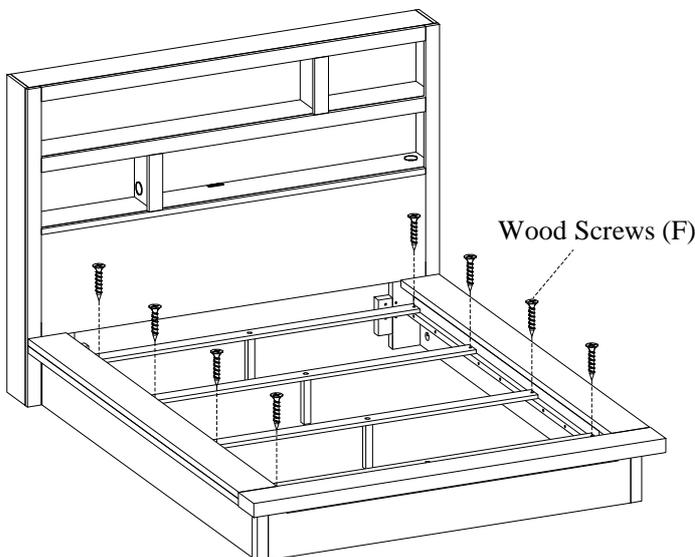
**STEP 3:** Arrange slats on the slat bearers and then lay the decking on top of the slats. Make sure the top and bottom slats are situated underneath the pre-drilled holes as shown below in STEP 4. Remove the decking and attach slats to the slat bearers with wood screws (F).
