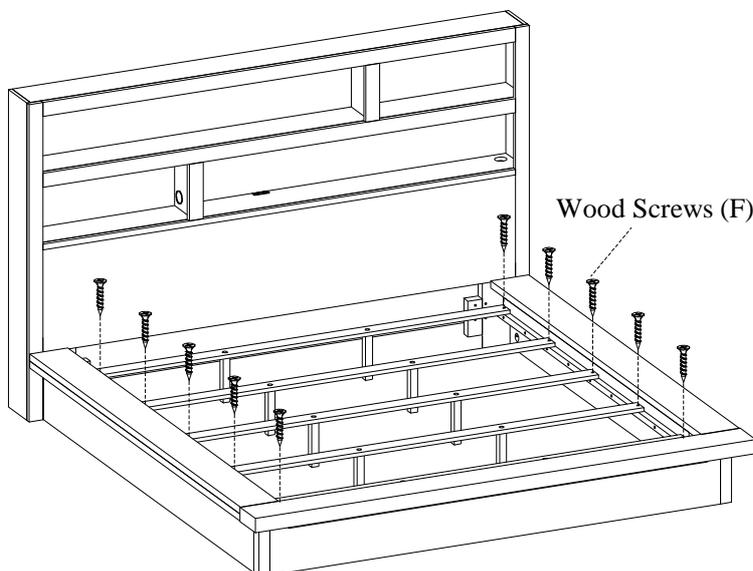
**STEP 3:** Arrange slats on the slat bearers and then lay the decking on top of the slats. Make sure the top and bottom slats are situated underneath the pre-drilled holes as shown below in STEP 4. Remove the decking and attach slats to the slat bearers with wood screws (F).
