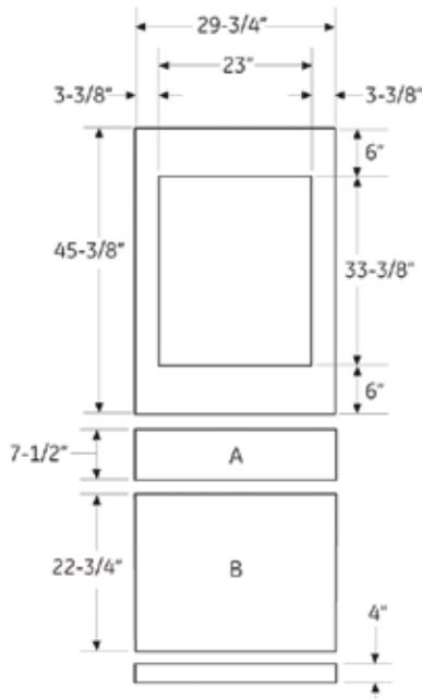
\*Styles must be a min 3-3/8" to cover aluminum door frame.
