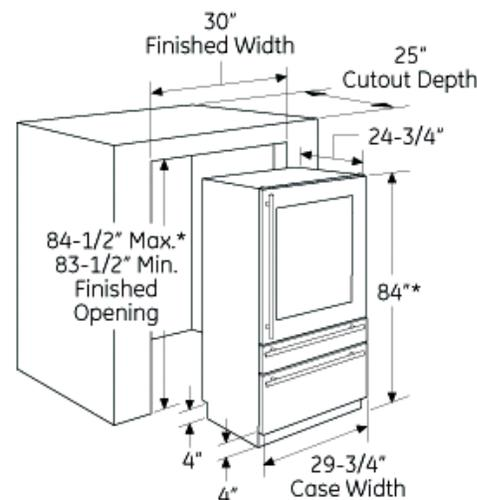
\* 84" high installation. The wine reserve can be adjusted to fit into a cutout that is 83-1/2" min. to 84-1/2" max. with the appropriate door kit. Use leveling legs and wheels for a maximum 1" height adjustment.
