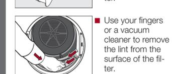
■ Use your fingers or a vacuum cleaner to remove the lint from the surface of the filter.
