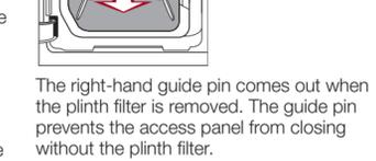
■ Push the plinth filter in completely. This will push in the right-hand guide pin at the same time.
