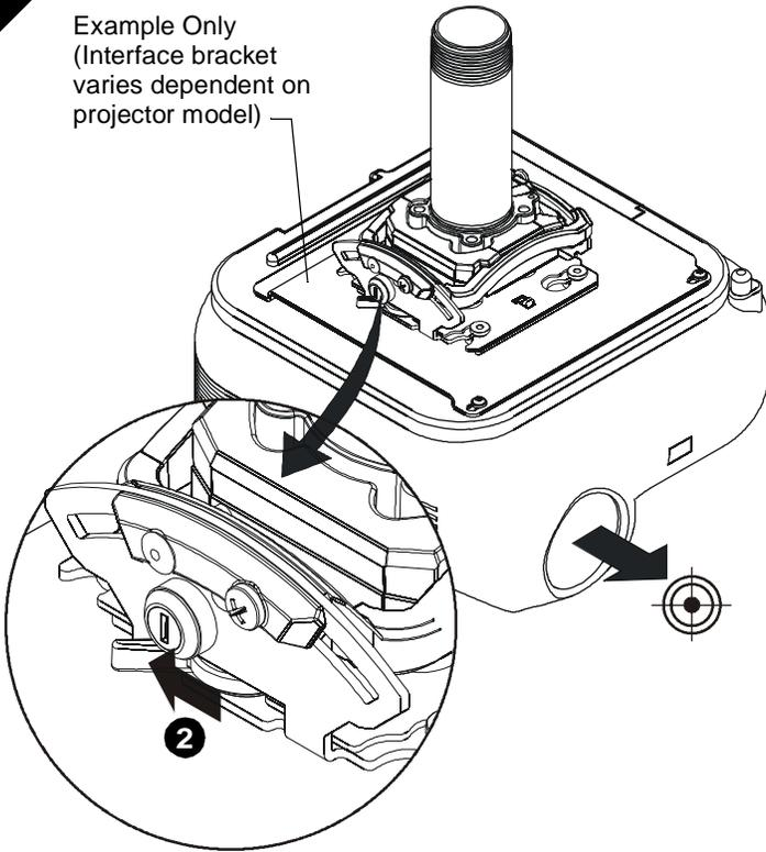
**Securing Projector with Interface Bracket to Model RSM Mount**
