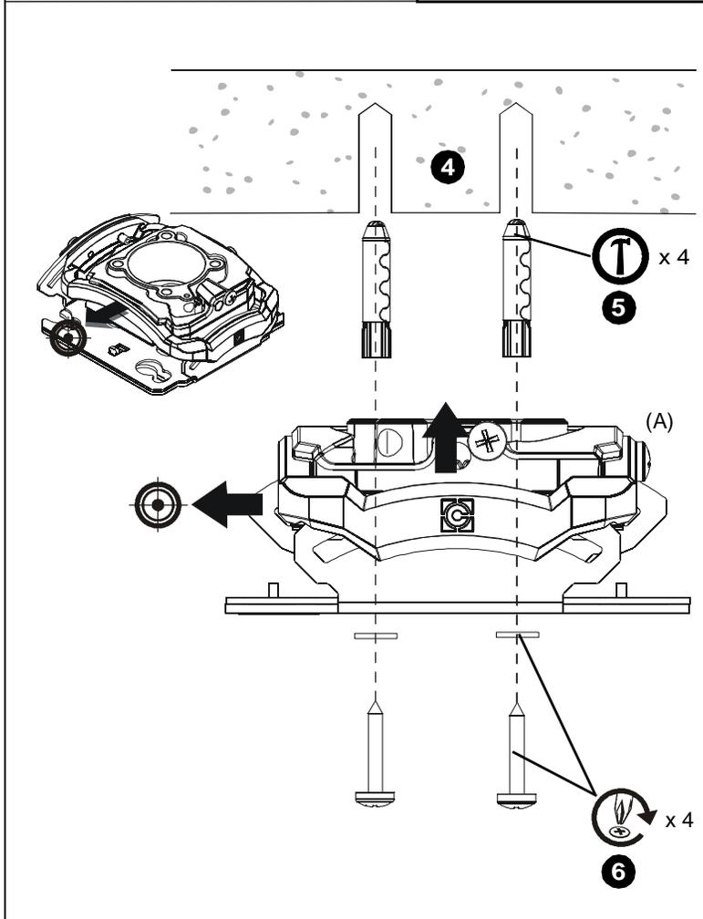
4. Align four mounting holes in RSM with four pilot holes.
