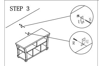
To insert the screw into each bracket and hang one on drywall anchor.
