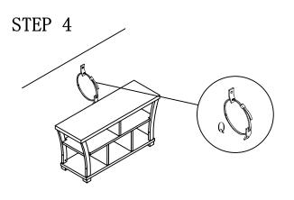
To tie the strap through bracket and pull it lightly till it steady.
