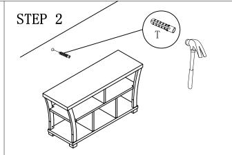
To tap drywall anchor into the hole.
