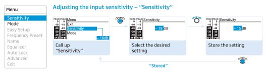
Adjustment range: 0 to -48 dB, adjustable in steps of 3 dB
