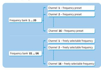
Each frequency range (A–E, G) offers 26 frequency banks with up to 16 channels each:
