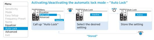
The lock mode prevents that the transmitter is accidentally switched off or programed during operation. The lock mode icon () on the standard display indicates that the lock mode is activated. For information on how to use the lock mode, refer to page 15.
