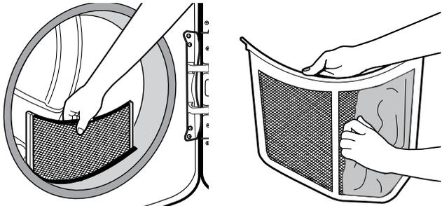
Clean the lint screen before each load. Pull the lint screen straight up. Roll lint off the screen with your fingers. Do not rinse or wash screen to remove lint. Wet lint is hard to remove. Push the lint screen firmly back into place.
