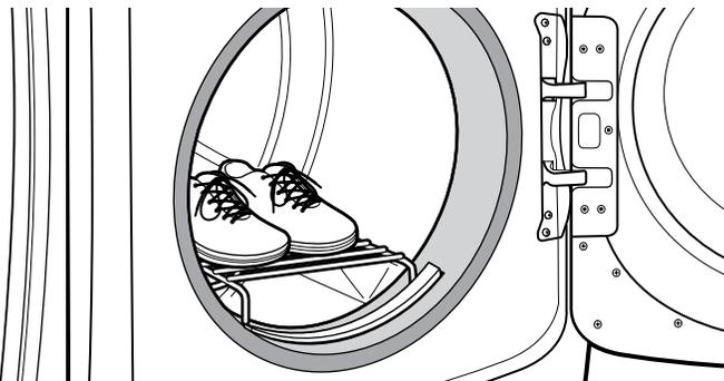
3. Place wet items on top of the drying rack. Allow space around items for air to circulate. The drying rack does not move, but the drum will rotate; be sure to leave adequate clearance between items and the inside of the dryer drum. Make sure items do not hang over the edges or between drying rack grille.
