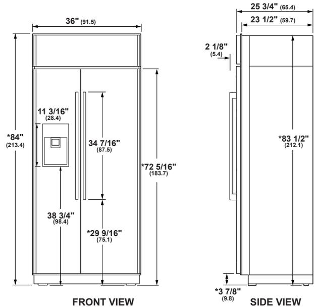
\* Shipping height. Use leveling legs and wheels for maximum 1" height adjustment from shipping height.
