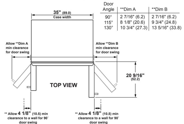
\*\* These refrigerators are equipped with a 3-position door stop. The factory-set 115° door swing can be adjusted to 90° if clearances to adjacent cabinets or walls is restricted. Allow full 130° door swings for pan removal. If the 90° door stop position is used, pan access is maintained, but pan removal is restricted.
