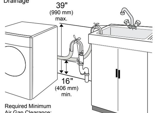
Required Minimum Air Gap Clearance:
