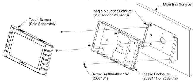
7. Secure the touch screen to the plastic enclosure with Phillip head screws. Alternatively, security Torx screws can be installed using a Torx screwdriver bit (both included with touch screen), as shown in illustration on page 8.
