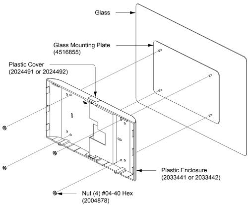
**NOTE:** When raceway is run to the bottom of the touch screen, the plastic cover must be placed in the top of the plastic enclosure. When raceway is run to the top of the touch screen, the plastic cover must be placed in the bottom of the plastic enclosure.
