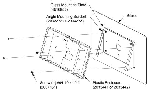
**NOTE:** When raceway is run to the bottom of the touch screen, the plastic cover must be placed in the top of the plastic enclosure. When raceway is run to the top of the touch screen, the plastic cover must be placed in the bottom of the plastic enclosure.
