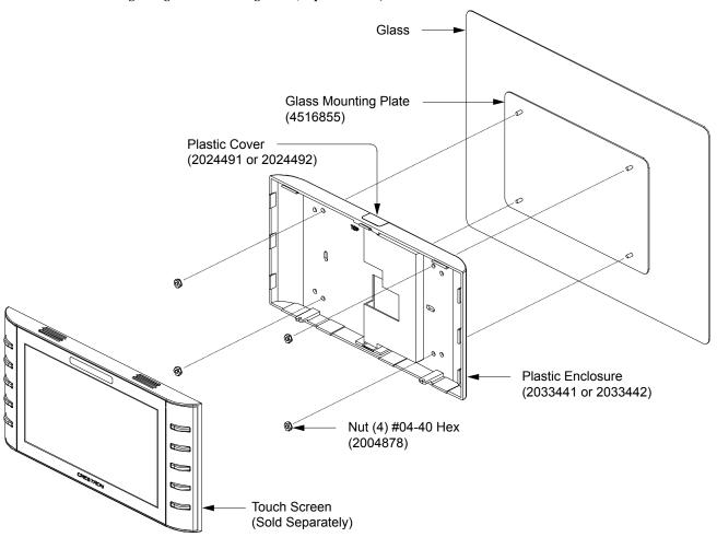
11. Secure the touch screen to the plastic enclosure with Phillips head screws. Alternatively, security Torx screws can be installed using a Torx screwdriver bit (both included with touch screen), as shown in the following illustration.
