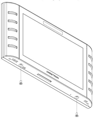
Secure Touch Screen with Screws (Mounting Surface Not Shown)
