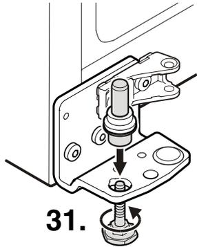
**31.** Tilt appliance slightly backwards, insert pin and attach using the adjustable foot.
