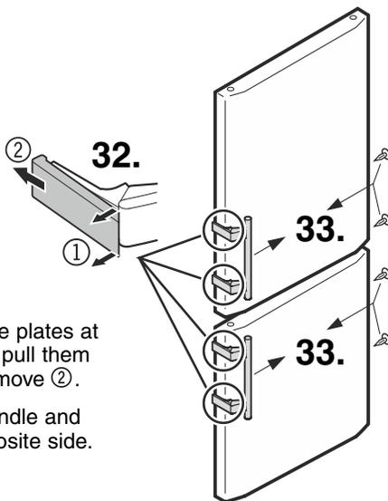
**32.** Release pressure plates at the front ① and pull them backwards to remove ②.
