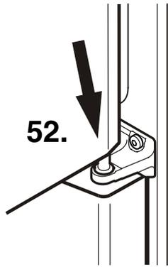
52. Suspend top door on hinge pin. For this, the door must be open at least 90°.
