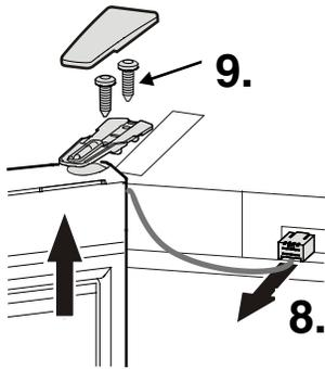
8. Disconnect the connector and pull the cable out of the guide.
