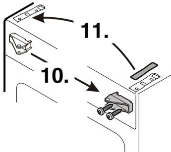
10. Transfer fastener for soft stop mechanism to the opposite side.
